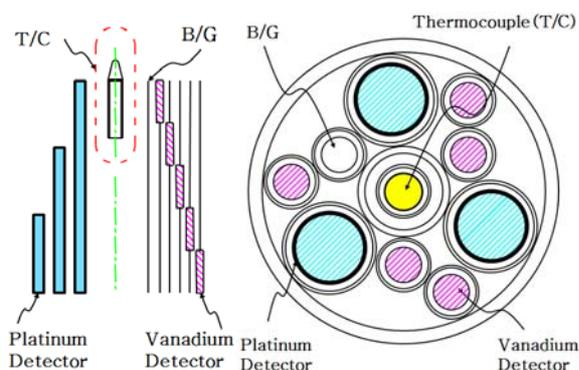
Figure 1. Axial and Radial Configuration
