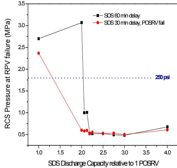
Figure 3. Depressurization performance according to SDS capacity in TLOFW
