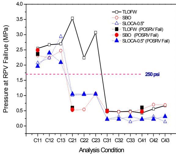
Figure 2. Depressurization performance according to SDS capacity and operation time
