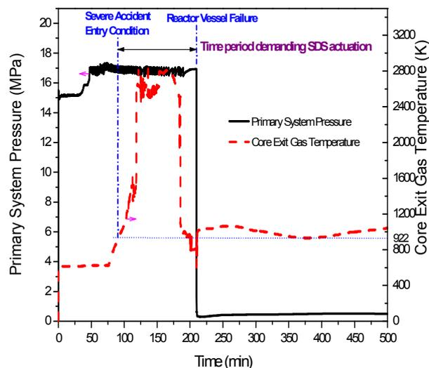
Figure 1. Analysis result of TLOFW with no ESFs
