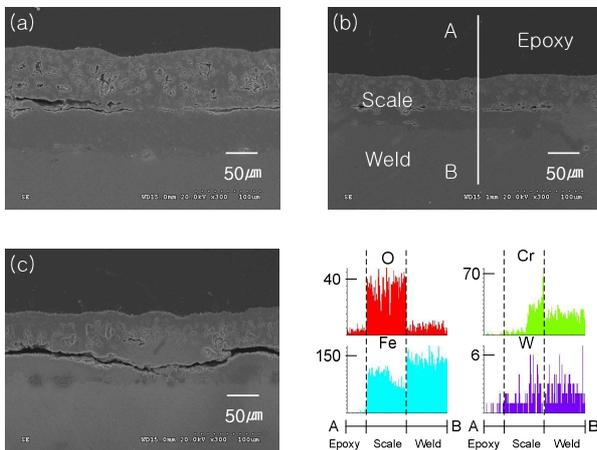
Fig. 3. Cross-sectional SEM images and EDS line profile of P92 steel after oxidation for 500hr at 700°C. (a) base metal image, (b) weld metal image, (c) HAZ image, (d) EDS of (b)
