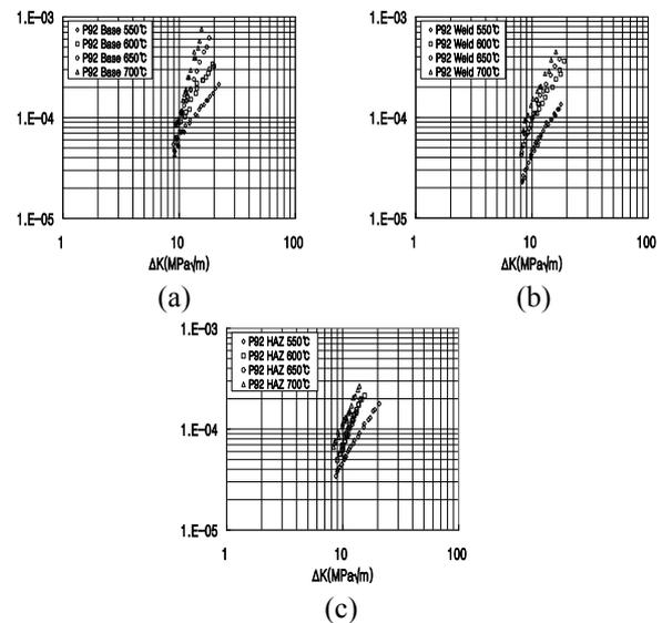
Fig. 4.  $da/dN$  vs.  $\Delta K$  curves in low  $\Delta K$  range (a) base metal (b) weld metal (c) HAZ.
