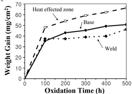
Fig. 2. Weight gain versus oxidation time curves of base metal, weld metal, and HAZ during oxidation at 700°C in air.
