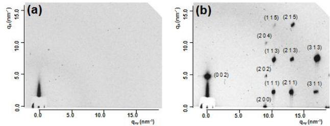
Fig. 3. Two dimensional GIXD patterns of (a) as-deposited rubrene film and (b) the crystalline rubrene thin films produced by abrupt heating at  $170 \text{ }^\circ\text{C}$  for 30 sec on electron-irradiated PS modified  $\text{SiO}_2$  (electron fluence:  $2 \times 10^{17} \text{ cm}^{-2}$ ).
