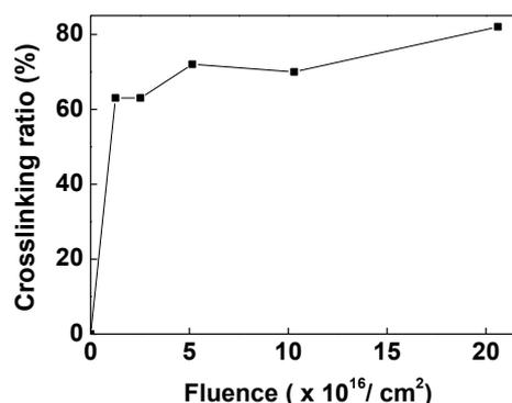
Fig. 1. Crosslinking ratio of polystyrene as function of electron irradiation dose
