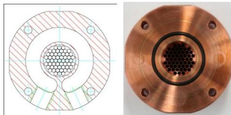
Fig.1. High yield  $^{11}\text{C}$  Target grid
