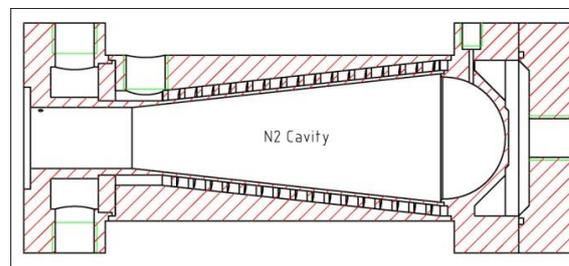
Fig.2. High yield  $^{11}\text{C}$  target  $\text{N}_2$  cavity
