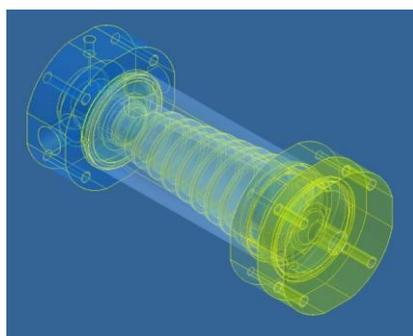
Fig.3. High yield <sup>11</sup>C target water cooling cavity
