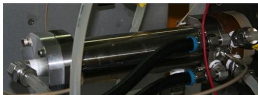
Fig.7. High yield <sup>11</sup>C target of KOTRON-13 cyclotron
