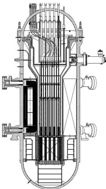
Fig. 1. The Layout of SMART
