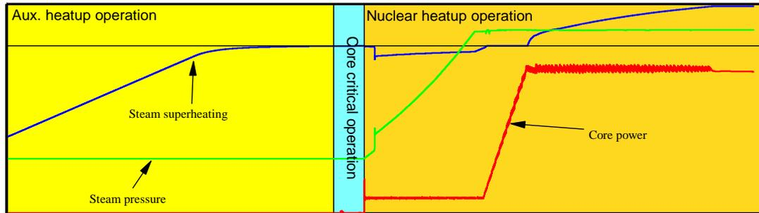
Fig. 4 Simulation of the startup operation of the SMART: Core power, secondary steam pressure and superheating
