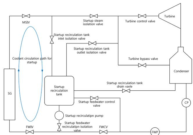
Fig. 2. Simple Diagram of SMART Secondary System
