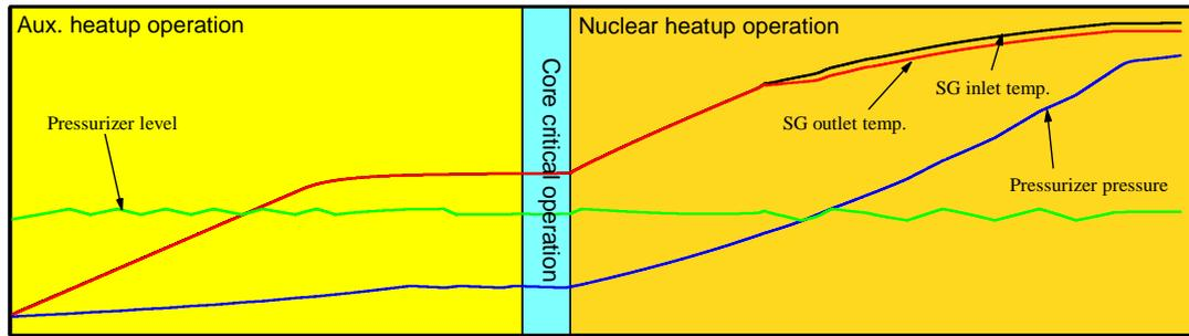
Fig. 3 Simulation of the startup operation of the SMART: Coolant temperature, Pressurizer pressure and level
