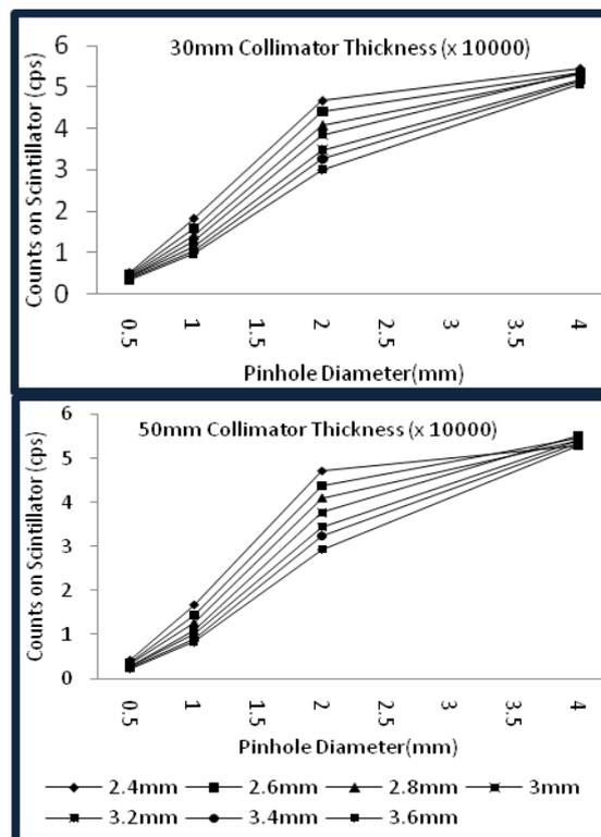
Fig 3. The number of photon depends on the diameter of pinhole and thickness of collimator counts are slower than before. This phenomenon appears when channel length is short and collimator thickness is thin. Moreover, the thicker collimator shows bigger difference of count rates by the channel length.
