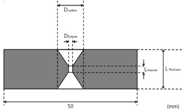
Fig. 1. Cross-section of collimator.
