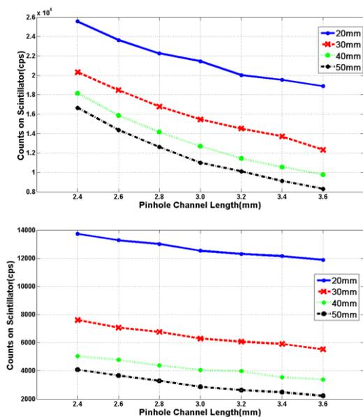
Fig. 2. 0.5 mm & 1 mm Count rate difference due to collimator thickness and channel length
