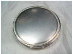
Fig.3 The fabricated prototype RI target (EB-welded)
