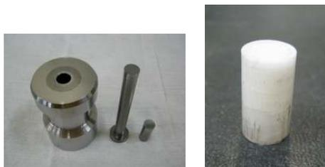
Fig. 4 Pressing of RbCl pellet
