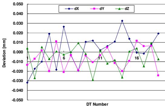
Fig. 5. Installation results of DT's center position for DTL106
