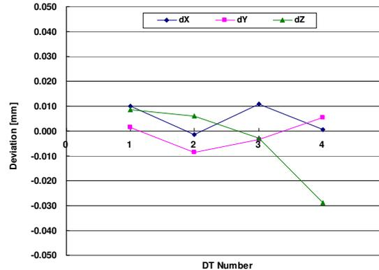
Fig. 7. Installation results of DT's center position for two MEBT tanks
