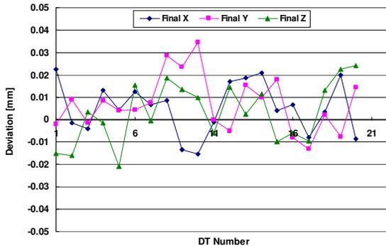
Fig. 4. Installation results of DT's center position for DTL105
