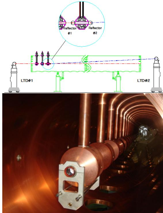
Fig. 2. Drift tube align procedure was accomplished with two laser trackers to real time position measurement.
