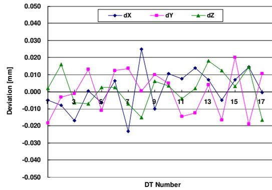
Fig. 6. Installation results of DT's center position for DTL107
