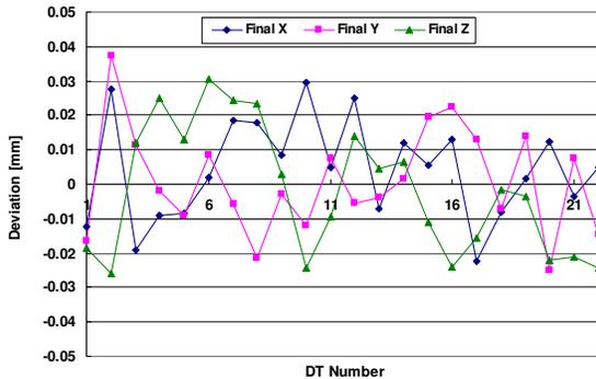
Fig. 3. Installation results of DT's center position for DTL104
