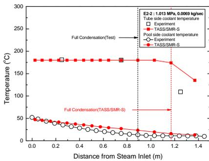
Fig. 3. Steam/coolant temperature at 1.0 MPa
