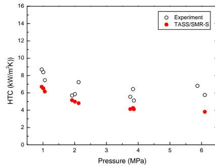
Fig. 7. Local condensation heat transfer coefficient by steam pressure
