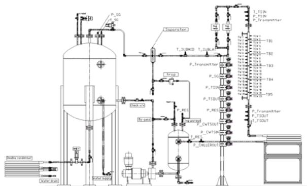
Fig. 1. Schematics of H/X tube heat transfer test
