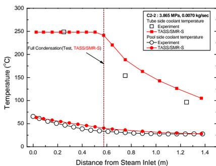
Fig. 5 Steam/coolant temperature at 4.0 MPa
