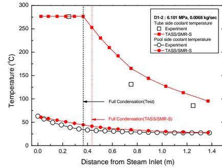
Fig. 6. Steam/coolant temperature at 6.0 MPa
