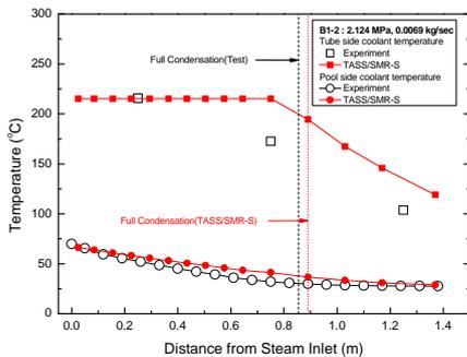
Fig. 4. Steam/coolant temperature at 2.0 MPa
