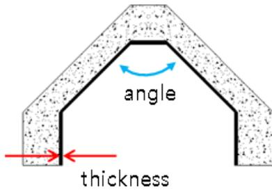
Fig. 3. Optimized X-ray target for electronic brachytherapy system or intra-cavity imaging.
