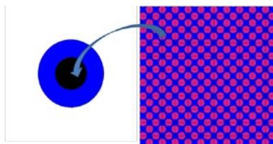
Fig. 4. MCNP Modeling of the Assumed Spherical Corium
