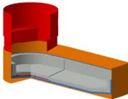
Fig. 1. A View of Core Catcher Developed in Korea
