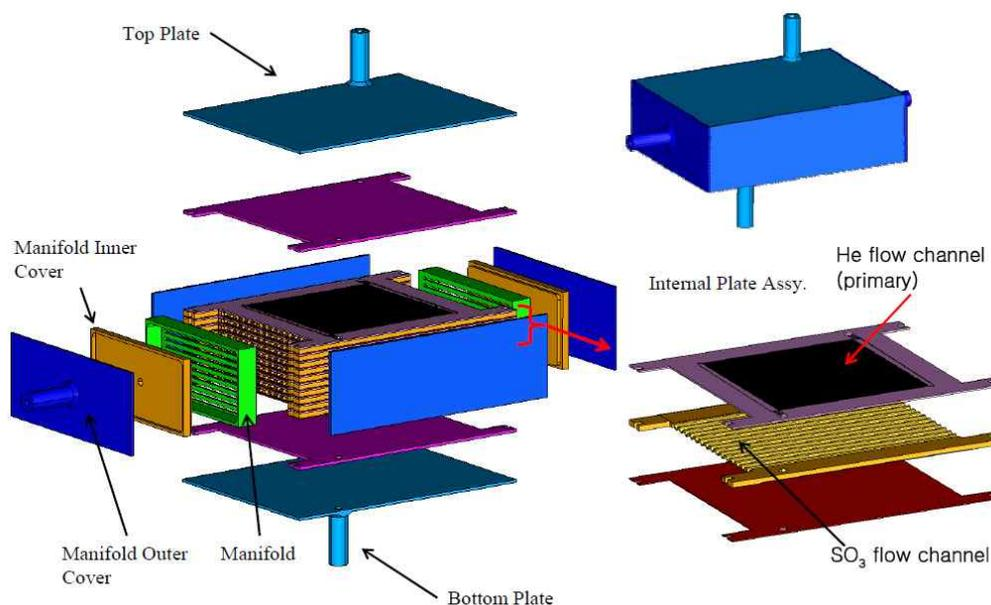
Figure 1 Drawing of Hybrid Heat Exchanger [6]
