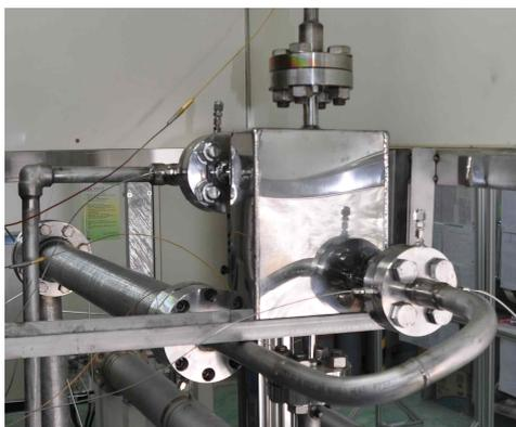
Figure 2 Installation of Hybrid Heat Exchanger
