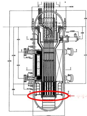
Fig. 1. Configuration of the SMART RPV and location of the beltline weld
