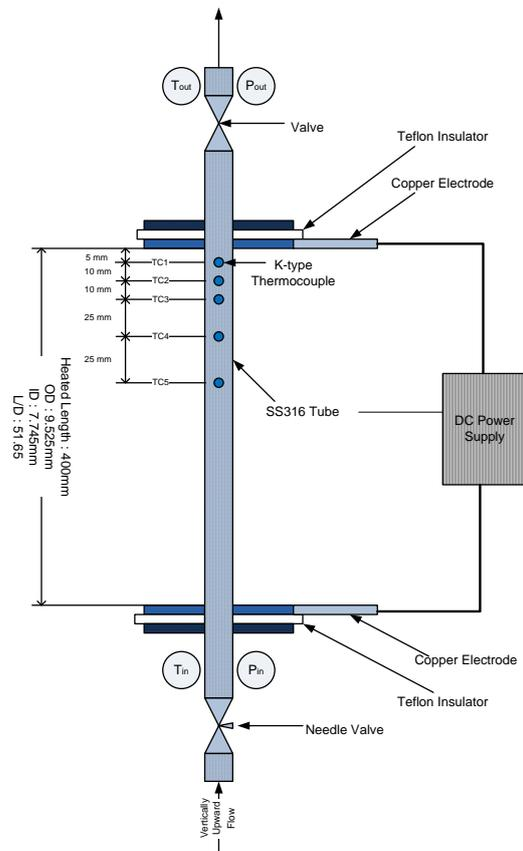
Figure 2. Schematic diagram of the test section
