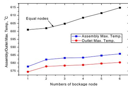
Fig. 3 Comparison of max. temp. with the blockage node numbers for the case that the reduced node size was applied to the central region
