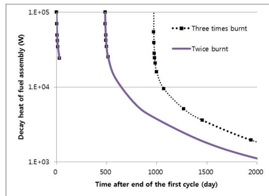
Fig.1 Decay heat of one fuel assembly
