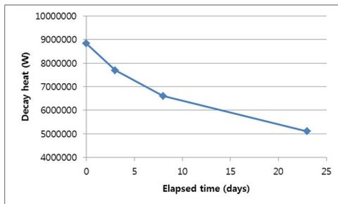
Fig.2. Decay heat of spent fuel storage pool
