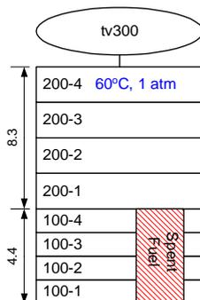
Fig. 3 MARS modeling of spent fuel storage
