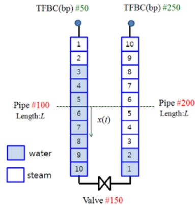
Fig. 3. Nodding diagram for oscillating manometers
