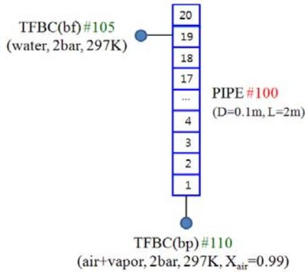
Fig. 1. Nodding diagram for falling liquid film tests
