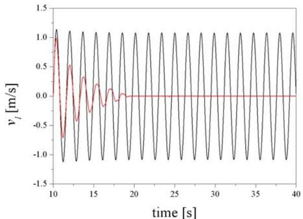
Fig. 4. Liquid velocities of case 1 (without wall drag: black line) and case 2 (with wall drag: red line)
