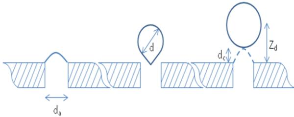
Fig. 1 Schematic diagram of bubble stream formation by P. Snabre(1997)
