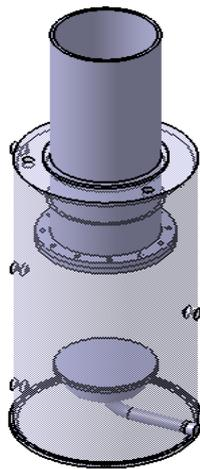
Fig. 2 Design of the test facility for bubble formation and velocity measurement
