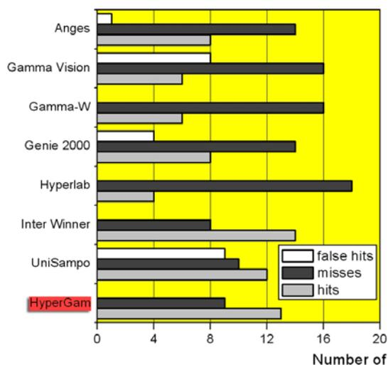
Fig. 1. Number of identified nuclides, misses and false hits in the MIX1EQ spectrum.
