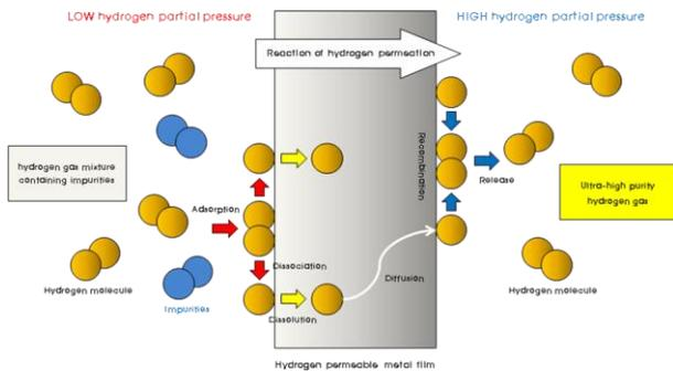
Fig. 1. The reaction of hydrogen permeation
