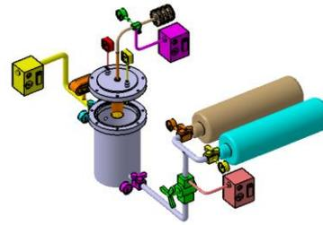
Fig. 5. The Schematic diagram of the experimental device.
