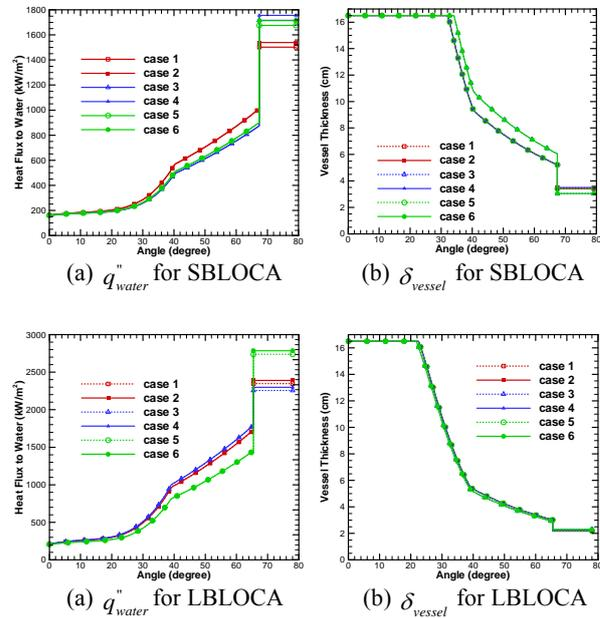
Fig 2 heat flux to water and vessel thickness for SBLOCA
