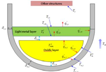
Fig 1 Schematic of the melt pool configuration in the lower head
