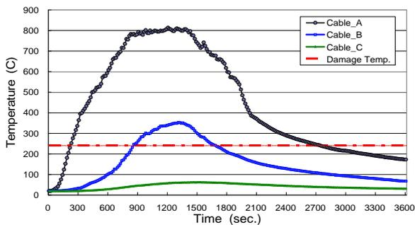
Fig. 2. Cable Temperatures in the Tray
