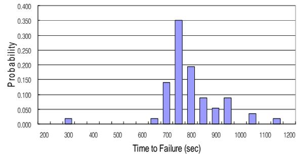
Fig. 4. Failure Probability of Cables in Tray B based on Damage Criterion (240C)
