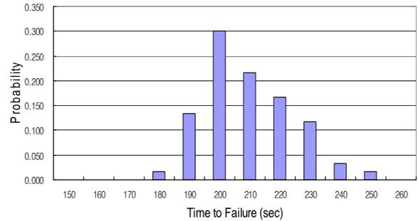
Fig. 3. Failure Probability of Cables in Tray A based on Damage Criterion (240C)
