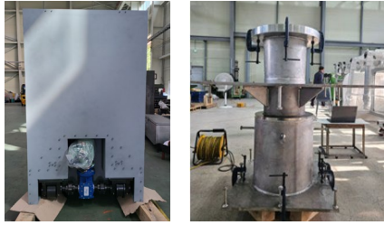
Fig. 3. Fabricated rear door frame and VMTS port for the FMPF hot cells
