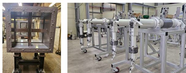
Fig. 2. Fabricated radiation shielding window wall liner and manipulator for the FMPF hot cells
