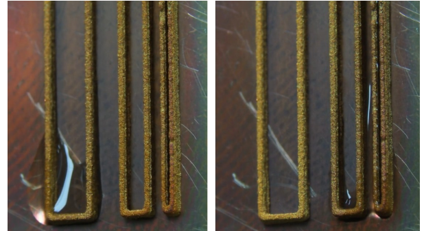
Fig. 2. Wicking test with water droplets (vertical channel)
