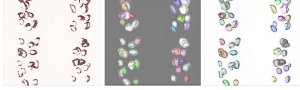
Fig. 9. Bubble detection stage (a) UNetL3 (b) Cellpose (c) ellipse fitting
