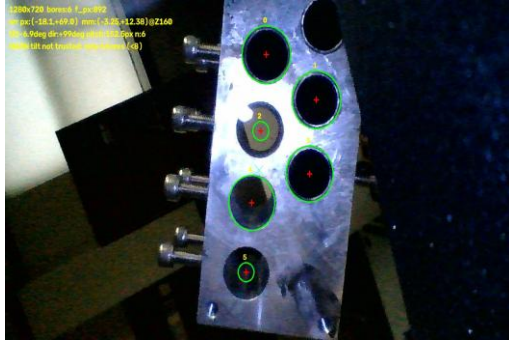
Fig. 2. Tube-sheet hole detection overlay from the onboard endoscope camera during the physical-mockup alignment test (measured data).
