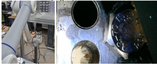
Fig. 3. Real-robot mockup test: (a) manipulator performing camera-based verification beneath the mockup tube sheet; (b) mockup bolt inserted into a tube-sheet hole.
