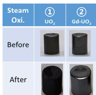
Fig. 2 Macroscopic appearances of conventional UO 2 and 8 wt.% Gd 2 O 3 -containing UO 2 pellets after steam oxidation at 1200°C.
