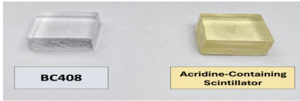
Fig. 1. BC408 and Acridine-containing scintillator with dimensions of 2 cm \times 2 cm \times 1 cm
