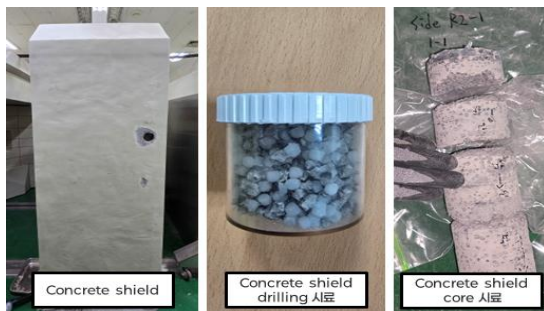
Fig. 1. Cyclotron concrete self-shield (Siemens Eclipse™)
