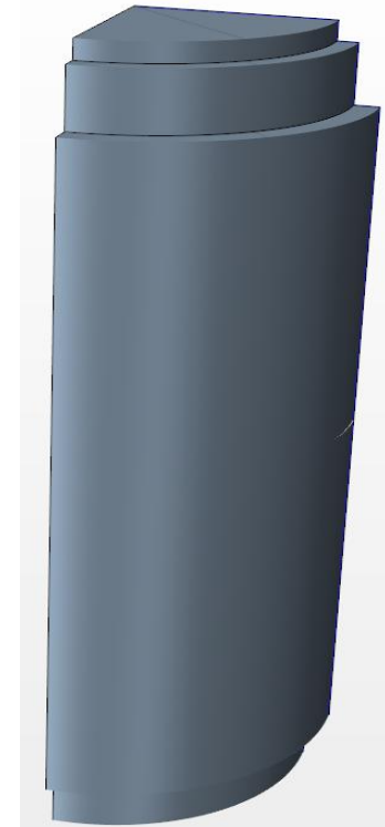
[Fig. 6. Quarter-symmetry computational domain of the TN-32B cask]
