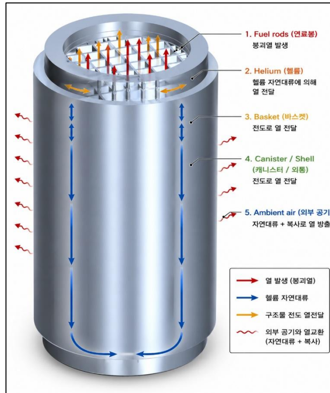
[Fig. 4. TN-32B cask configuration and major heat removal paths]
