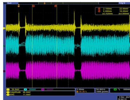
Fig. 1. Snapshot of DPO 4034 display showing the gated measurement interval for reflected RF power acquisition.
