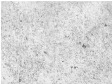
Figure 5 Vertical surface of the compact pressed at 170 °C and subsequently heat-treated
