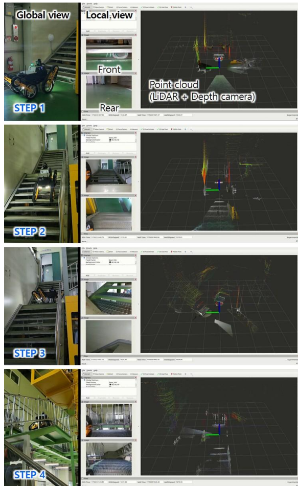
Fig. 4. Sequential steps (STEP 1 to 4) of a stair climbing experiment with global and local view data
