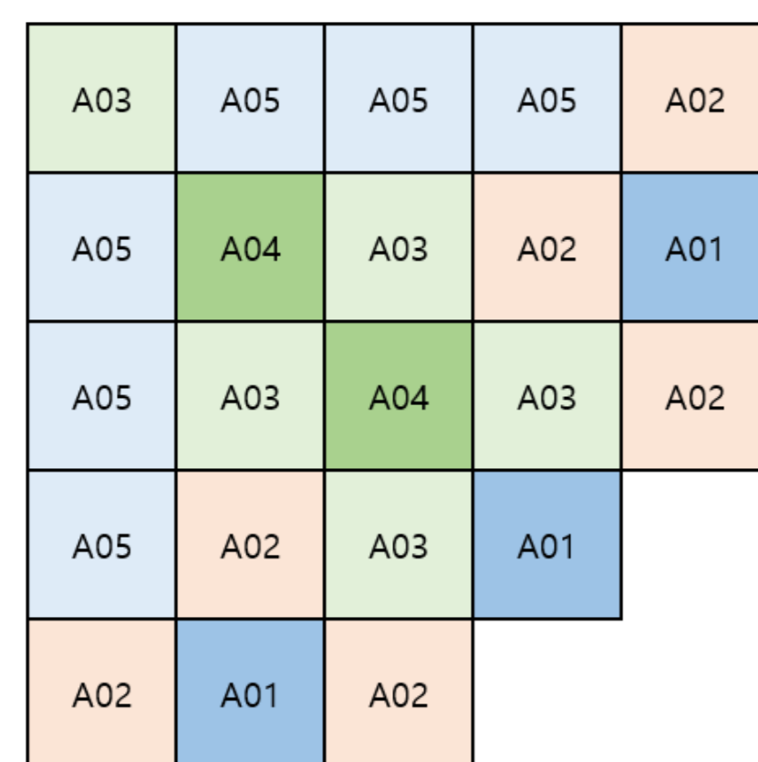
Fig.1 Loading pattern of the i-SMR core
