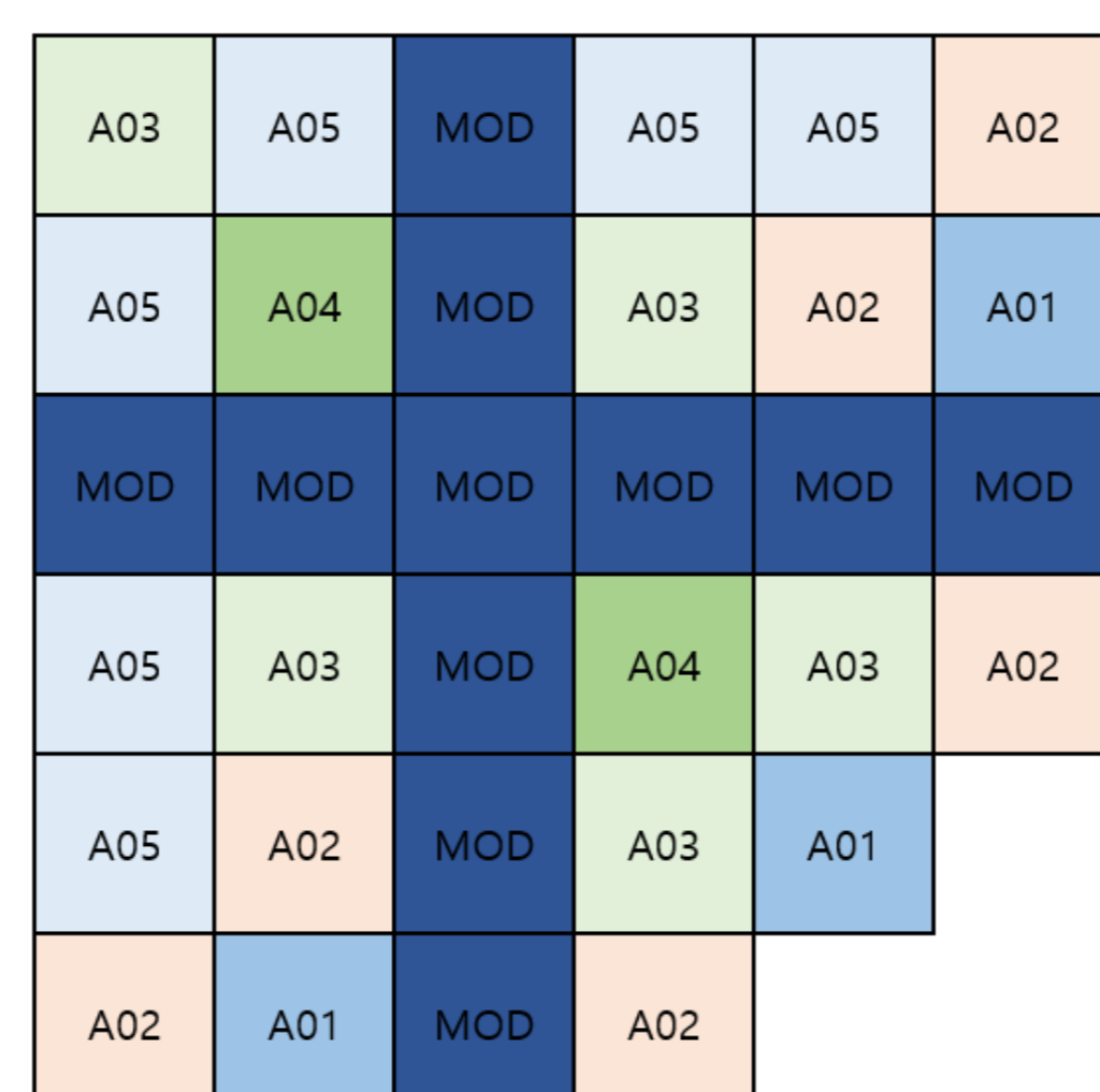
Fig.5 Loading pattern implementing the assembly spacing based reactivity reduction concept
