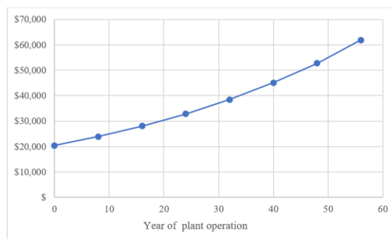
Figure 4. Increase in solenoid valve replacement cost over a 60-year plant lifetime
