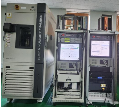
Fig. 1. Experimental configuration of the accelerated aging test for safety-related digital input cards.
