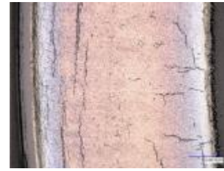
Fig. 1. PIE-reported radial hydrides in spent-fuel cladding under normal operating conditions (adapted from [2], with permission).
