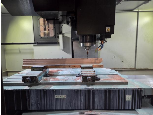
Fig. 3. RFQ minor vane under final machining.
