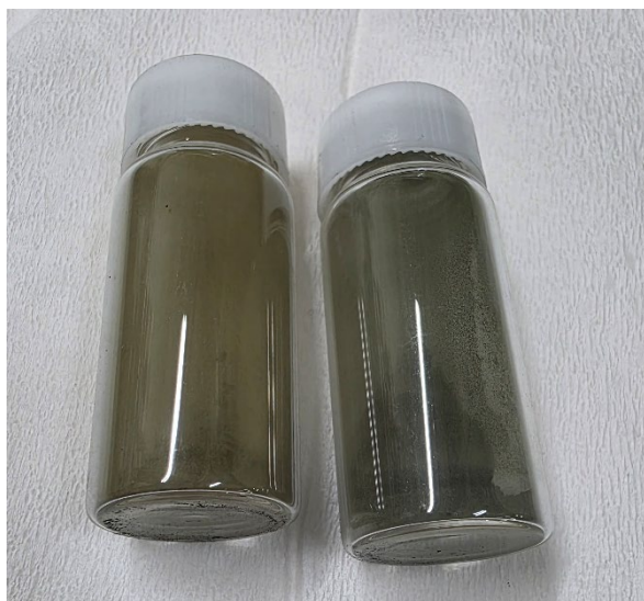
Fig. 3. Reaction products obtained from the BiCl 3 -based chlorination of uranium: UCl 3 (left) and UCl 4 (right)
