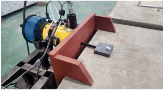
Fig. 2. Test set-up for shear test
