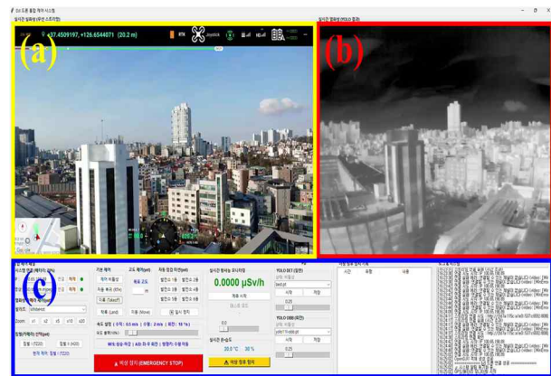
Fig. 4. Designed real time monitoring layout of the integrated monitoring GUI, simultaneously displaying (a) visual streaming, (b) thermal streaming, and (c) the control panel.
