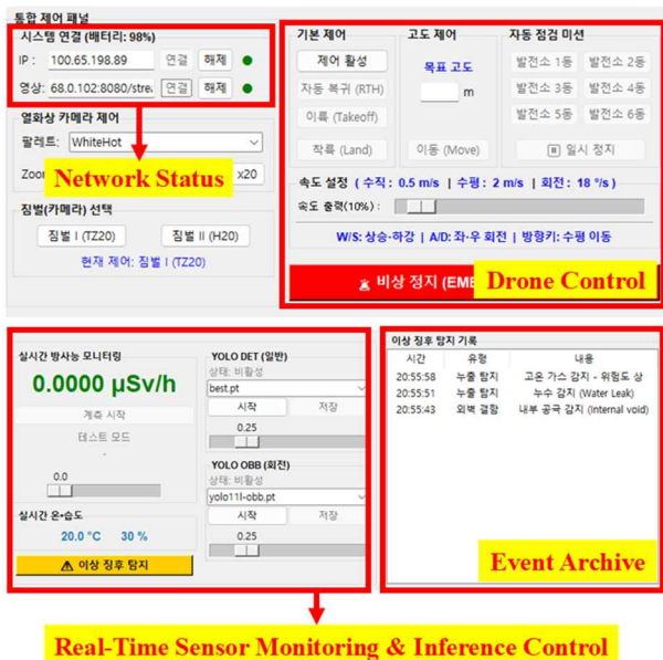
Fig. 3. Detailed functional layout of the control panel, illustrating components for network status, flight control, real-time sensor monitoring, inference settings, and event archiving.
