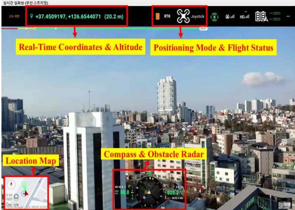
Fig. 2. Detailed view of the visual streaming interface with native MSDK OSD widgets, displaying essential flight metrics and adaptive navigation data.
