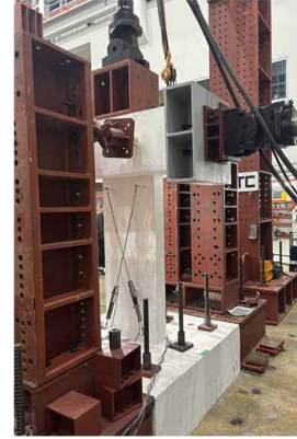
Fig. 2. Hybrid simulation model of NPP auxiliary building. Among seven stories, where the first story is set as an experimental substructure.
