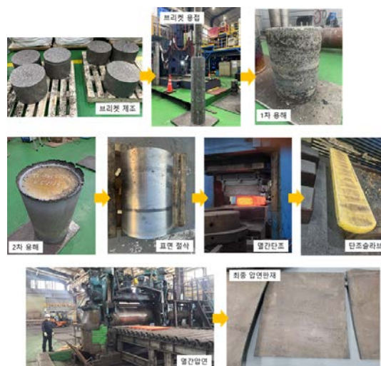
Fig. 1. Fabrication routes for industrial scale titanium-based neutron absorbing structural material
