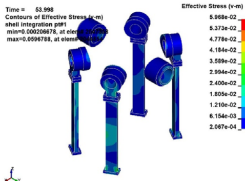
Fig. 4. The von-Mises stress contour of the RPV [6]
