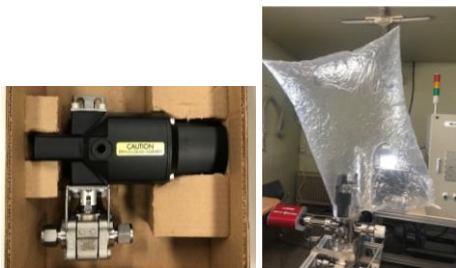
Fig. 2. Helium leak test for one of candidate ball valve: Swagelok S60P steam service.
