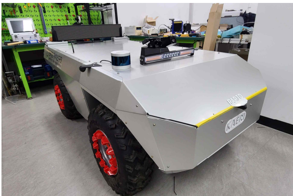
Fig. 1. The developed unmanned ground vehicle for prevention of radioactive disasters by providing outdoor radiation information in nuclear facility
