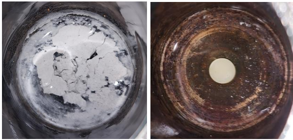
Fig. 2. Autoclave test results on pure \text{Gd}_2\text{O}_3 and 15at.% \text{CeO}_2 doped \text{Gd}_2\text{O}_3
