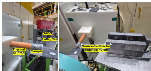
Fig 1. Experimental setup for the performance evaluation of scintillation detectors.
