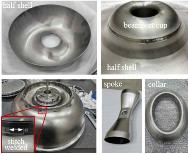
Fig. 2. Each part consisting the single spoke resonator cavity
